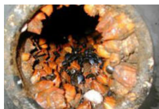
▲ Eroded water pipe due to the propagation of marine organisms
